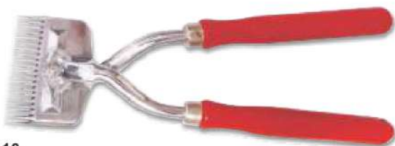
40-108-10 Hand sheep clipper with wooden handle
